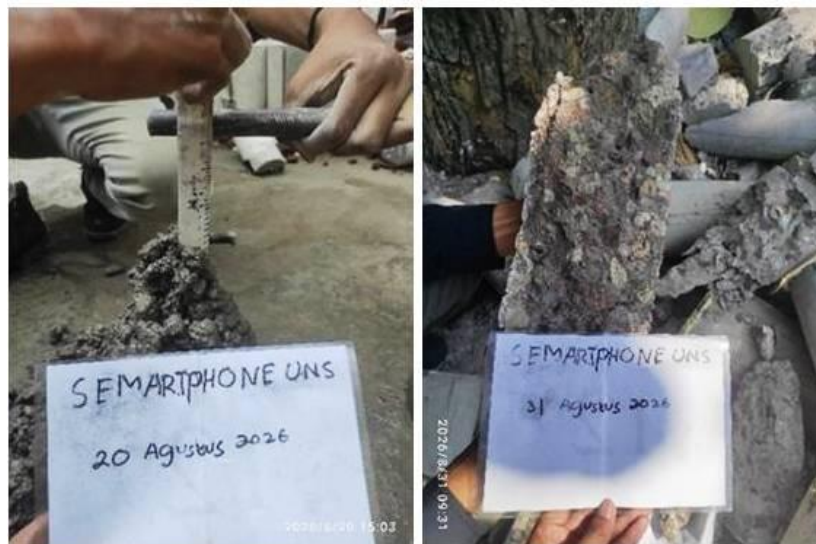
Figure 3. Slump Test and Concrete Sample Appearance after Compression Test
