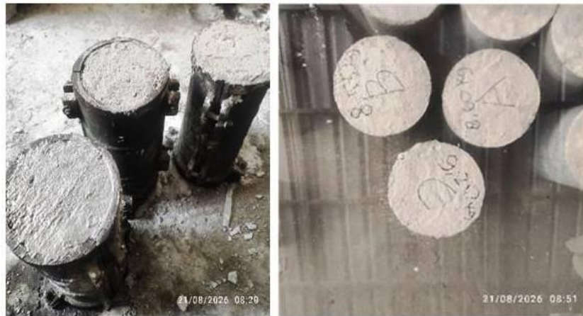
Figure 2. Sample Preparations and Curing Process
